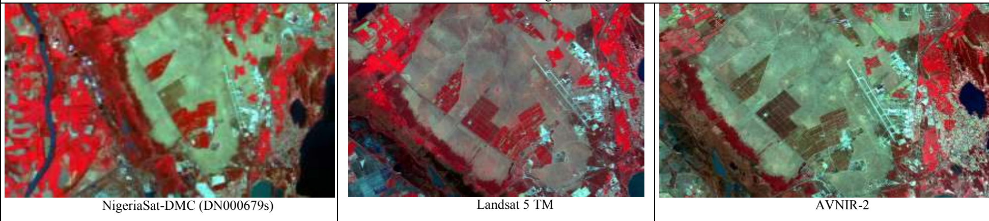
Blurred artefact on DMC image. The contrast of TM image composition is better than the DMC one.
