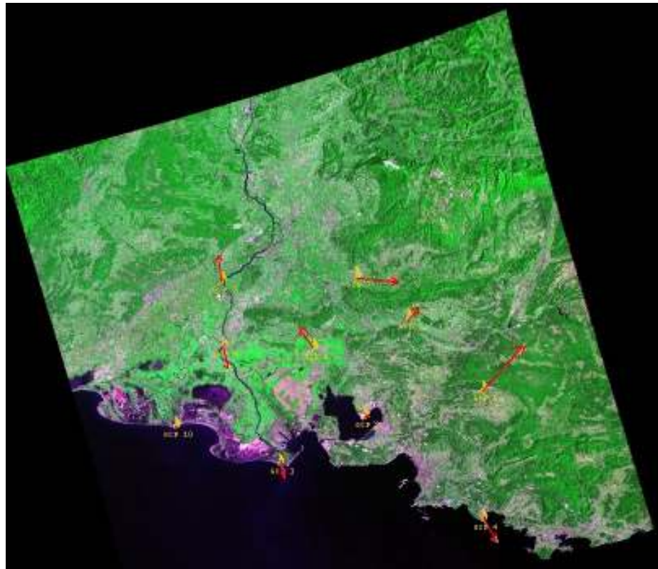
fig. 11 - Planimetric accuracy results (m), DN00067bp, UK DMC (Vector magnification X300).
