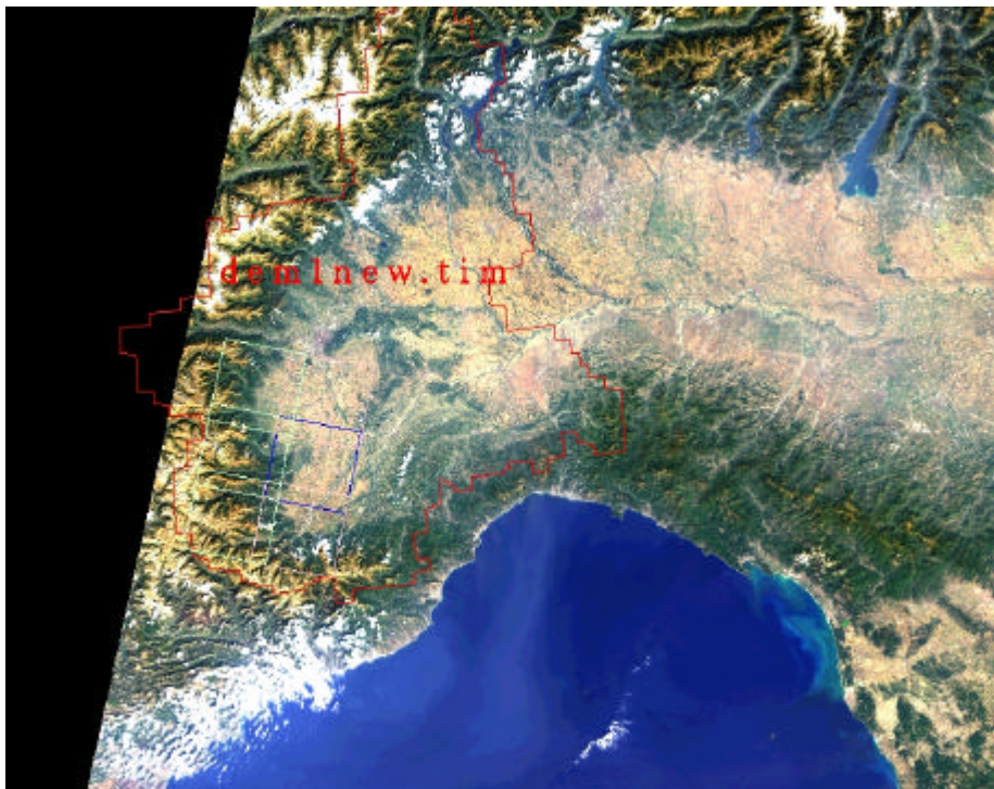
fig. 11 - DEM 50 m resolution boundaries (red) for Piemont test site superimposed over MERIS-FR image.
